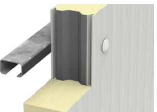
Recommended for rooms with positive temperatures and not below 4°C. In case of rooms with temperatures below 4°C it is appropriate to carry out a thermohygrometric analysis of joint permeability, which might affect the efficiency of the cold room and cause issues of condensation and/or ice formation. The joint geometry is tongue-and-groove interlock and the panel is fitted with standard PU/PE gasket inserted during production, hence no additional on-site work steps are required.
