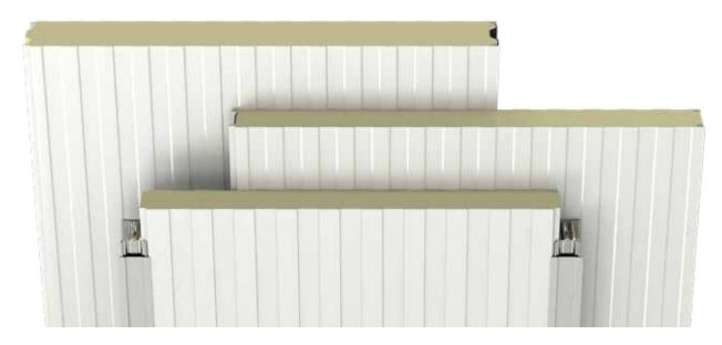
The Isopan Cold Solutions product range includes sandwich panels with a tongue-and-groove labyrinth joint and gasket, with double metal facing and polyurethane foam insulation with a high insulating capacity.
