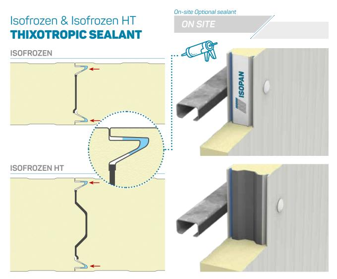
Recommended for negative temperature rooms; the thixotropic behaviour of the sealant enables a simple and quick assembly with excellent air tightness thanks to the lack of cracks. The sealant is added inside the cavity of the female side, along the entire length of the panel, by using a dosing gun.
