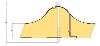
The proper screw length depends on panel thickness and on the type of support (steel, wood).
