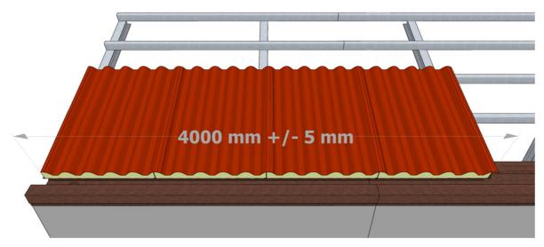
Note: take care to properly place the panels during the assembly step (4 panels =  $4000 \text{ mm} \pm 5 \text{ mm}$ ) in order to prevent problems during the next ridge installation step, as shown in the figure.
