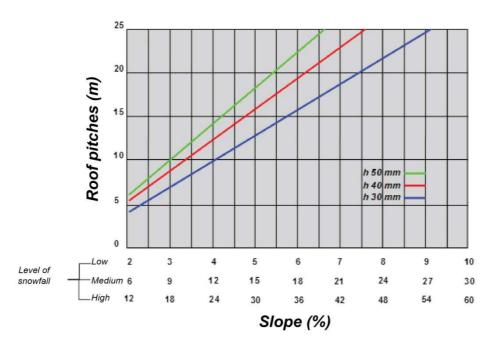
In the former case, the minimum slope, in relation to the climatic area and the rib height, can be taken from the **Slope diagram**. We recommend (in the event of low or average level of snowfall) a slope no less than 7%.
